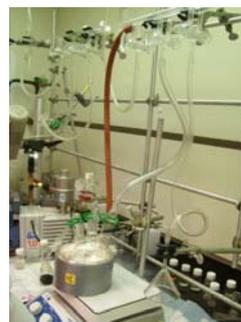
Synthesis of technetium sulfides
