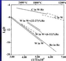
The minimum coefficient of diffusion  $D$  is typical of self-diffusion of W and Re and the tracer diffusion of refractory  $Me$  (Re, Ta, Mo, and Nb) in W.
