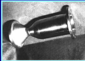
450 N chamber. Starting material Re rod Ø 110 mm
